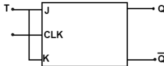
Figure 6: T Flip Flop Using JK Flip Flop
